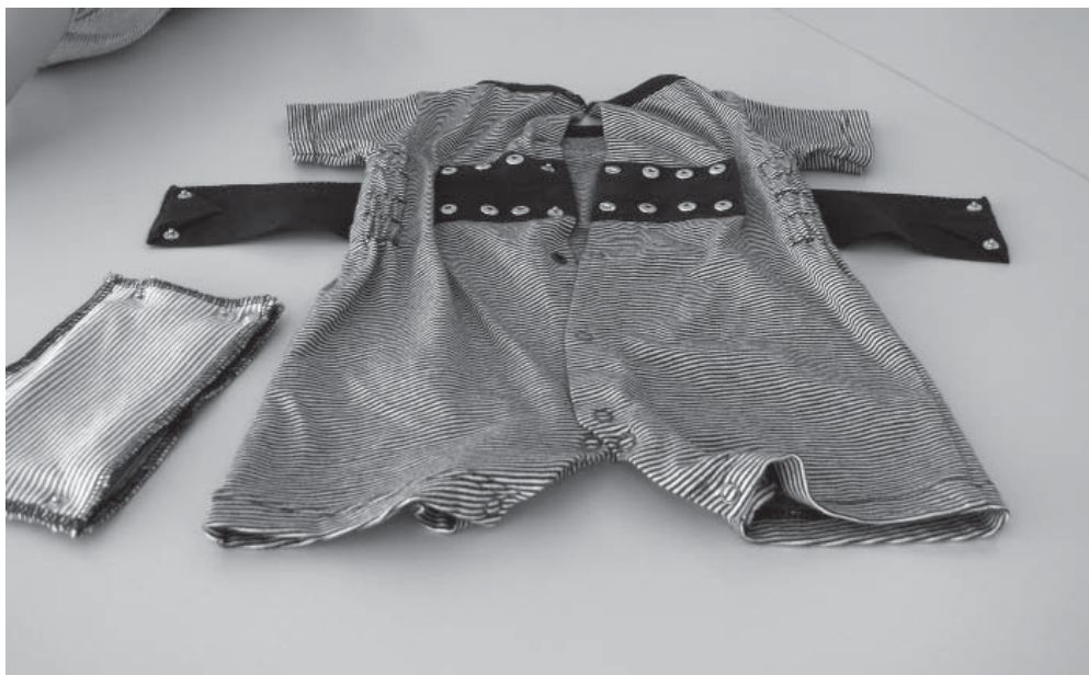
Fitted to a romper suit, the stretchable printed circuit board monitors infants' breathing. (© VERHAERT Masters in Innovation®) | Picture in color and printing quality: www.fraunhofer.de/press
